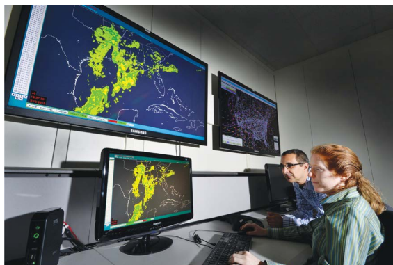
Figure 11. The Offshore Precipitation Capability provides a real-time depiction of weather beyond the range of radars, filling in key coverage gaps in the Gulf of Mexico, the Caribbean, and other regions.
