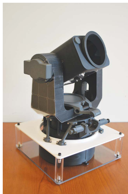
Figure 5. Engineering model of a laser communications terminal.
